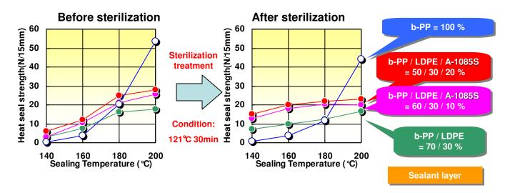
Structure: Sealant (20 μ m) / Substrate (b-PP 50 μ m) // DL // PET(24 μ m) b-PP : PP impact copolymer DL: Dry Lamination
